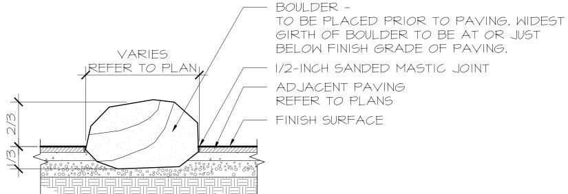
GIRTH OF BOULDER TO BE AT OR JUST BELOW FINISH GRADE OF PAVING. - 1/2-INCH SANDED MASTIC JOINT --- ADJACENT PAVING REFER TO PLANS - FINISH SURFACE
